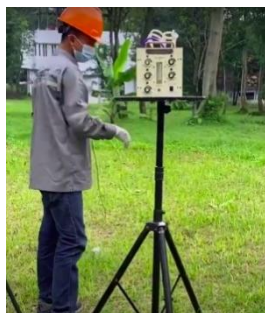
Ambient CO Measurement Using a CO Meter
